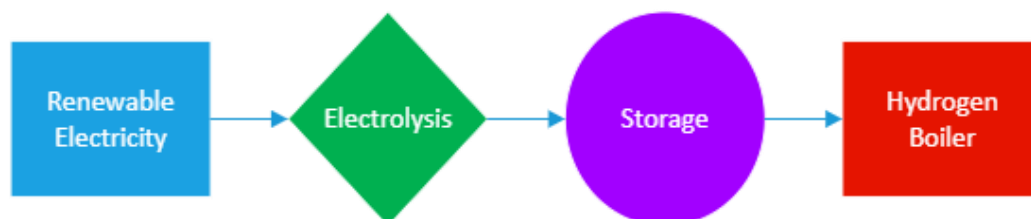
Figure 9: Simplified flow of hydrogen for substituting fossil fuels in a cement production process
