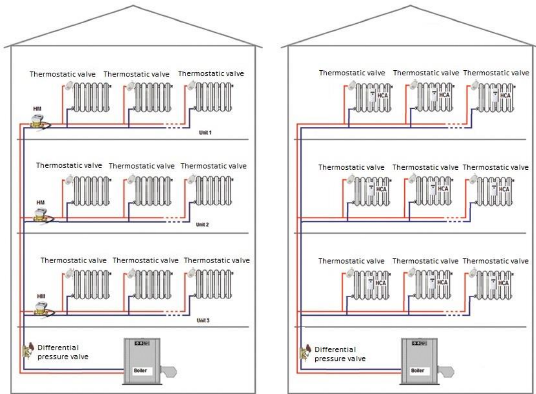
Figure 10: a) Reference buildings' central heating system with heat meters, b) Reference buildings' central heating system with heat cost allocators
