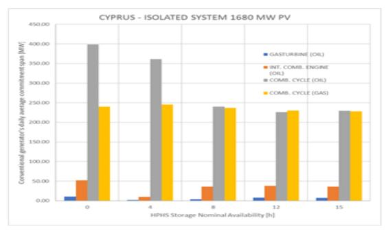
Results for the 275 MW PHS system were summarized  $\rightarrow$  The 0h value is for the case where no PHS system is installed
